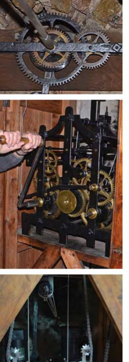
down to the ground level. The hourly strike mechanism originally operated using a hammer striking the Tenor bell via a series of pulleys, levers and wires.
